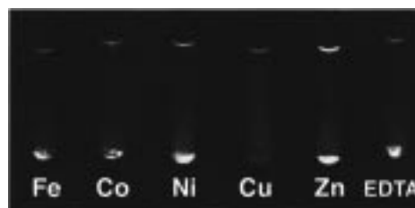
Figure 3. Typical solid-phase quenching assay of 5 . The samples shown are in 50 mM Hepes, 150 mM NaCl, and 10% v/v methanol (pH 7.0) and contain 100 \mu M of the appropriate divalent metal cation or EDTA. Fluorescence excitation was provided with a handheld low-wattage mineral lamp set on “long wavelength” (365 nm). The image was acquired after 2 h of incubation.
